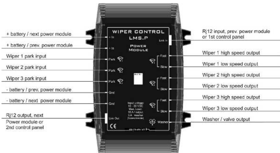
Picture 3.2: 'Power module front view'
